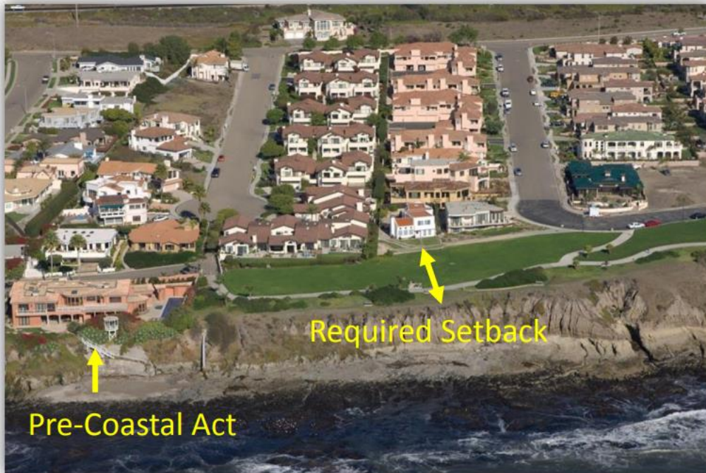
Figure 18. Photo depicting a development setback in Pismo Beach. (Source: California Coastal Records Project )
